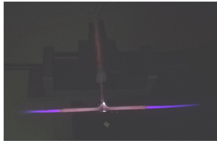
Figure 4 Plasma-Gun: Generation of a "volumic" plasma at atmospheric pressure in a T-tube
