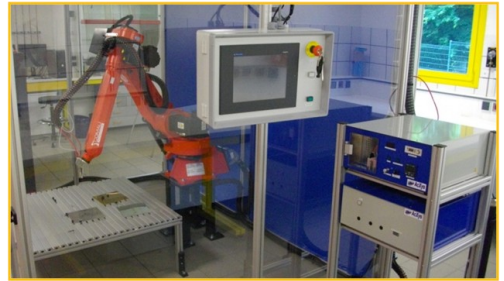
Figure 2 - Acxys® Atmospheric Pressure Plasma Torch on Six Axis Robot
