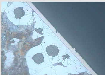
Nickel deposit on a cast G x 100 Thickness of deposit : 16 \mu m
