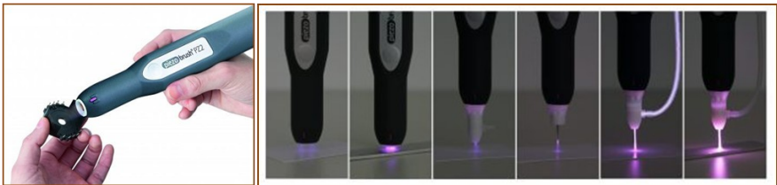
Figure 3 Manual Torch (Piezobrush® PZ2 from Relyon Plasma GmbH) with different nozzles
